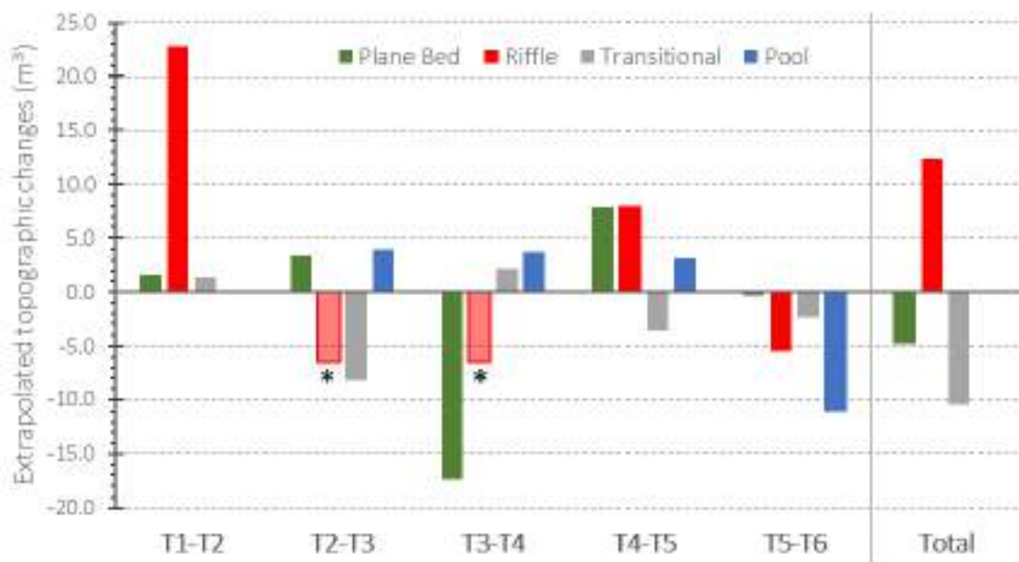
Figure 5.12. Topographic changes (net) in the upper River Ehen, extrapolated from changes in cross-sectional area (only changes above the minimum level of detection have been considered, see methods). See Figure 5.1 for details on the morphological units. Note that there was no suitable topography data for T3 at the riffle, therefore for T2-T3 and T3-T4: the value of T2-T4 is divided between the two (Indicated with *).
