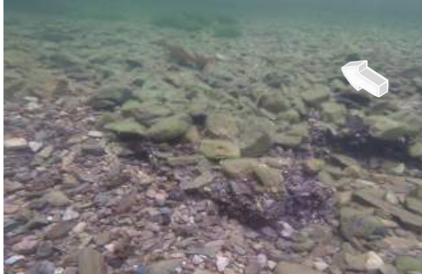
Plate 7.1. Photographic evidence of partial break-up of the pavement downstream from a hydraulic jump. Arrow shows flow direction. (Photo: Baptiste Marteau).
