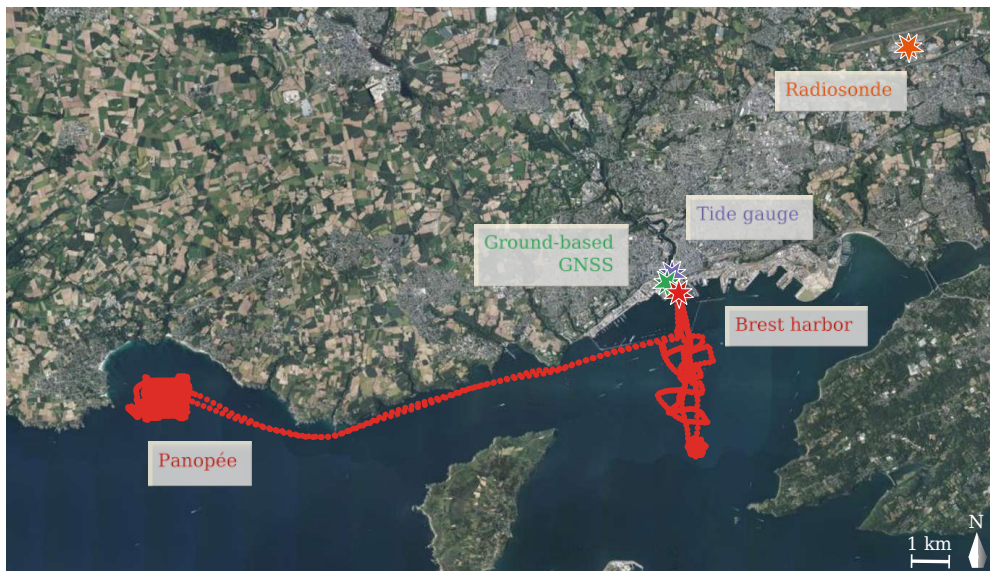
Figure 4.2: Map of the Bay of Brest with the Panopée course between days 89 and 137 of 2018 (red), and the locations of Brest ground-based GNSS station (green), nearby Penfeld tide gauge (purple), and RS station of Météo France in Guipavas (orange). Panopée is docked in the Marina du Chateau (red star) most of the time, which is next to the tide gauge and the ground-based GNSS antenna. This map was created thanks to QGIS.
