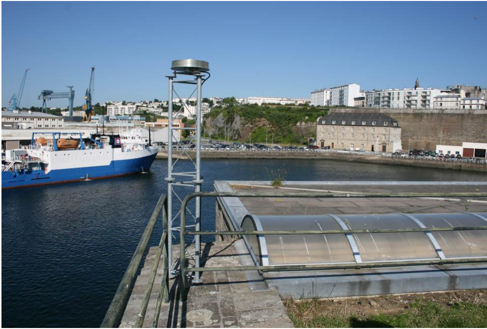
Figure 4.7: Photo of the BRST antenna located in the Penfeld estuary. (Retrieved from igs.org - Accessed October, 25th, 2023).
