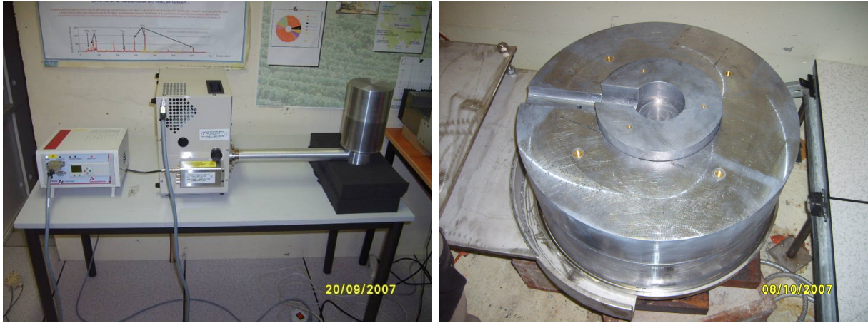
Figure 3.5: Mafalda, the planar low background HPGe for gamma spectrometry installed at LSM. Left: the detector endcap, the cold finger and the pulse tube. Right: lead shielding.
