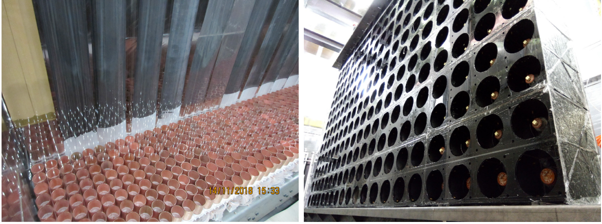
Figure 1.13: Left: Source foils and tracker in SuperNEMO demonstrator. Right: calorimeter wall
