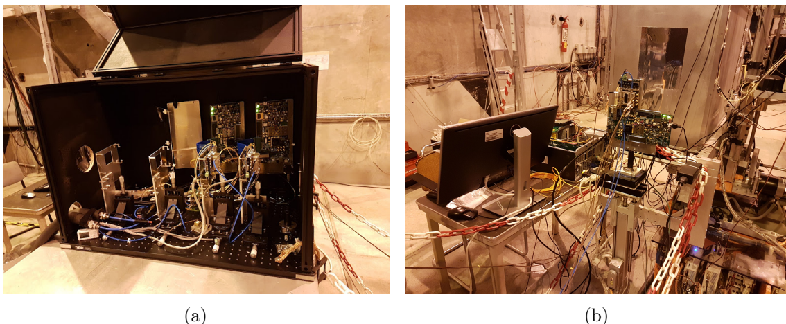
Figure 5.11.: 5.11a : The box with planes 1 and 2 of TDCPix, close together. Picture taken during the test beam in 2017. 5.11b : The TimePix3 telescope (gray box) and plane 3 of TDCPix ("L" structure in front of it). Picture taken during the test beam in 2017.
