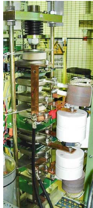
Figure 5-26.- Arrangement of the switching cells and clamp circuit components of the IGCT set-up
