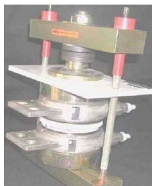
Figure 1-32.- Press pack diode arrangement
