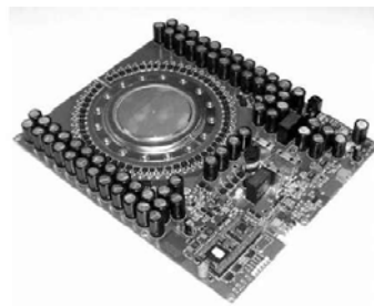
Figure 1-36.- 38mm IGCT sample with experimental gate unit for test purposes
