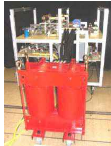
Figure 2-22.- Test bench mechanical assembly arrangement Figure 2-23.- Output inductor disposition.
