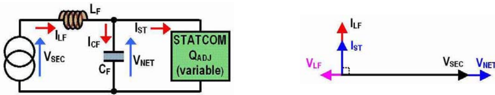
Figure 4-34.- System steady-state vector diagram considering the input filter L_F , C_F
