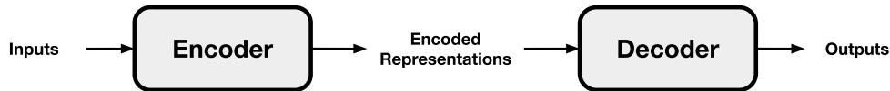
FIGURE 2.2: Encoder Decoder Networks which embeds the input to an intermediary representation which gets decoded by the decoder to final representation.
