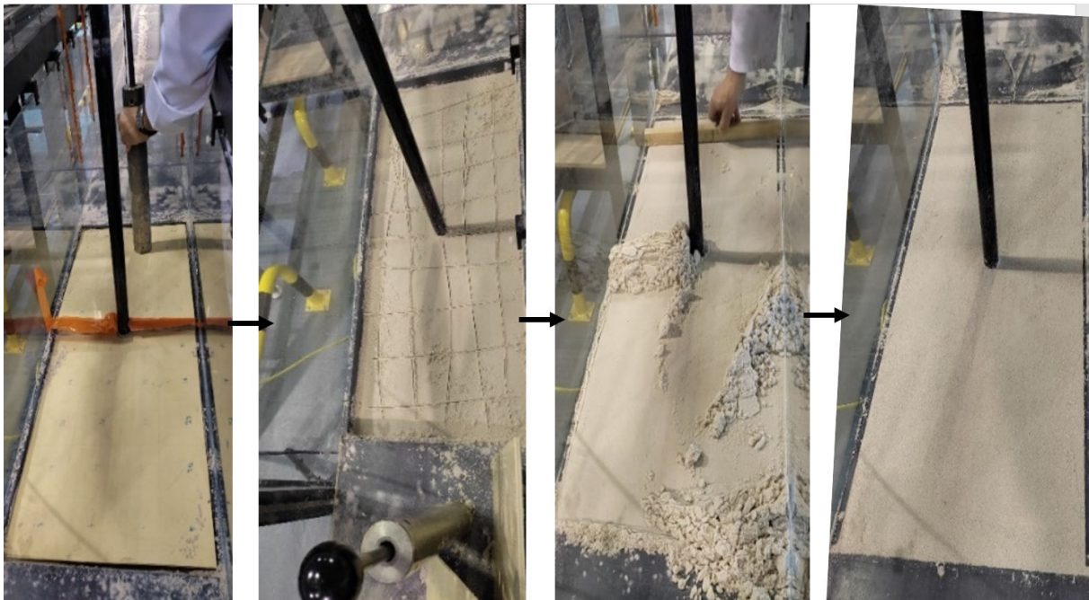
Figure II.20: Procedure for placing the soil in the flume
