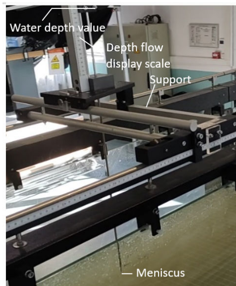
Figure II.10: Manual Level Gauge
