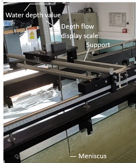
Figure II.10: Manual Level Gauge
