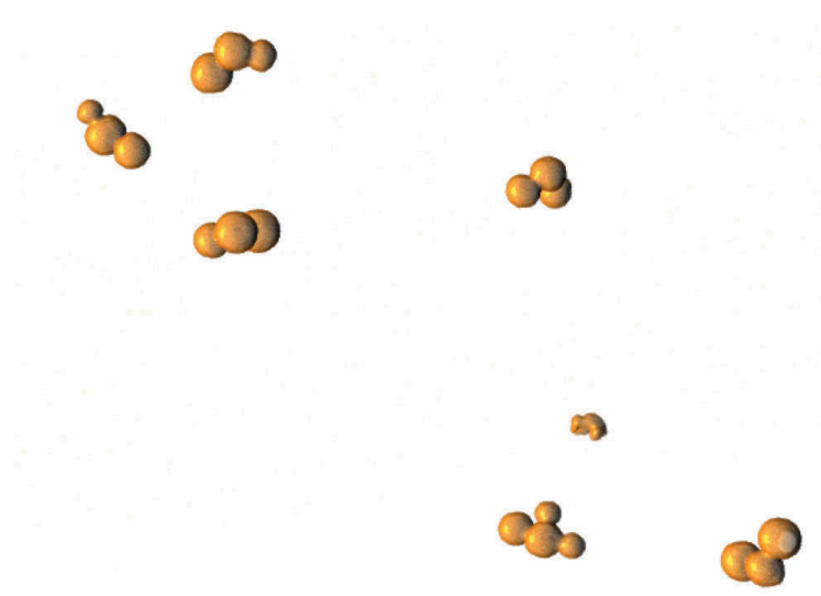
Figure 16. Merged pores inducing low sphericities (adhesive B, high temperature curing).
