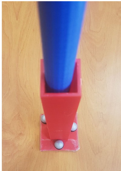
Figure 4.17: Close-up look on the red square hole and blue peg used for the peg insertion task. The square hole is 2.25 cm x 2.25 cm wide and the peg diameter is 1.9 cm
