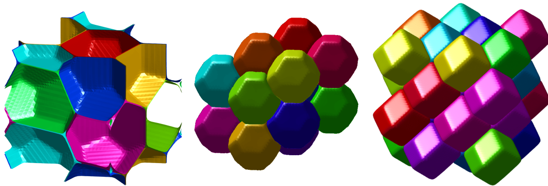
Figure 4.18: Some computations on the periodic cube: the Weaire-Phelan structure for n = 8 , the Kelvin structure for n = 16 and the rhombic dodecahedron structure for n = 32 .
