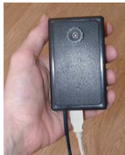
Fig. 1. The complete camera whose thickness is about 2cm.
