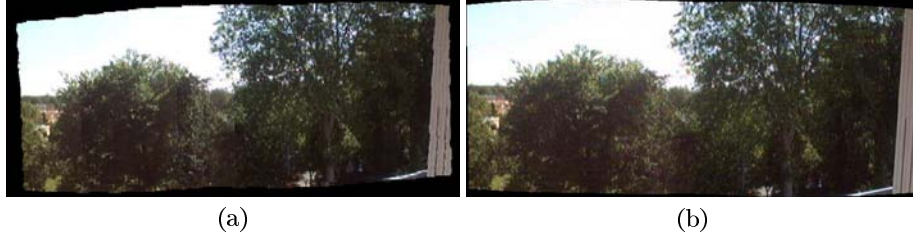
Fig. 4. (a) A part of the panorama from 4 images before the bundle adjustment and post processing. (b) The same part after refinement and post processing.
