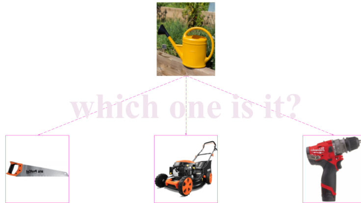
Figure 1.3: Illustration of the challenges of product retrieval for an online hardware store. (i) The query image is a picture of a watering can taken in its natural environment, while all catalog images are taken on a clean white background. (ii) The class "watering can" does not appear in the catalog.
