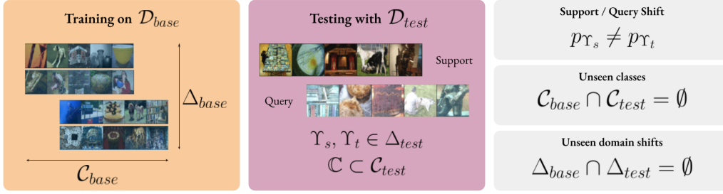
Figure 3.2: A Few-Shot Learning algorithm is trained on a base set \mathcal{D}_{base} made of images from a set of domains \Delta_{base} and labels from a set of classes \mathcal{C}_{base} . At test-time, the trained model is fed with a support set sampled from a new (source) domain \Upsilon_s \in \Delta_{test} and new classes \mathbb{C} \subset \mathcal{C}_{test} and is asked to classify query samples from another (target) domain \Upsilon_t with p_{\Upsilon_t} \neq p_{\Upsilon_s} . Importantly, both classes and domain shifts are not seen during training ( \mathcal{C}_{base} \cap \mathcal{C}_{test} = \Delta_{base} \cap \Delta_{test} = \emptyset ), making Few-Shot Learning under Support-Query Shift a challenging problem of generalization.
