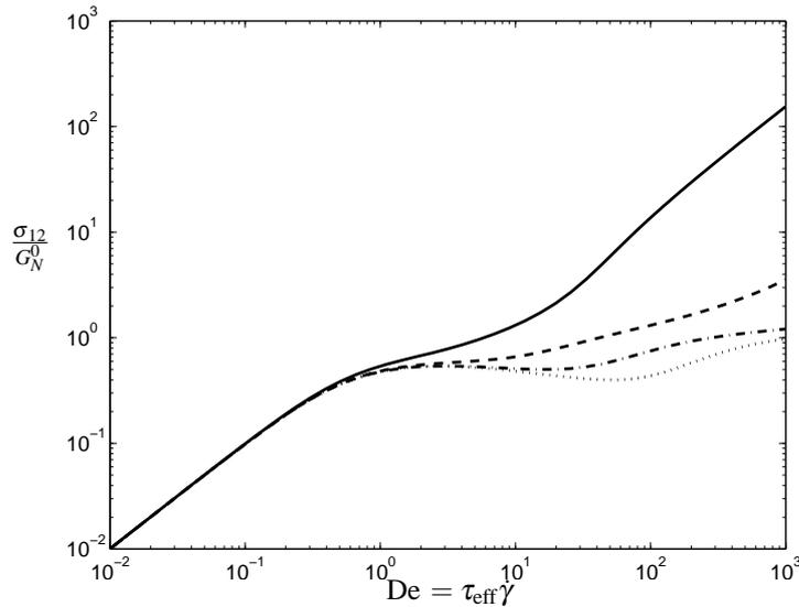
Figure 3.2: Steady state shear stress as a function of the Deborah number. The four curves correspond to different  $\tau_d/\tau_r$  ratios (—: ratio= 10, - - : ratio= 30, - · - : ratio= 100, · · · : ratio= 300).
