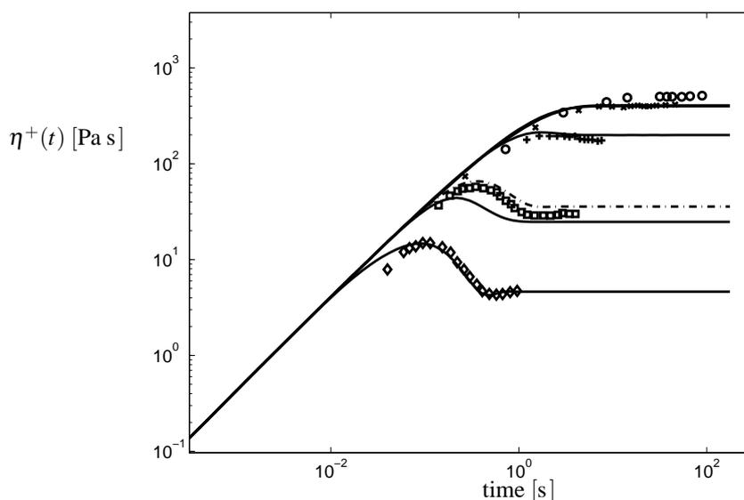
Figure 3.8: Transient shear viscosity for S1. Comparison between experimental results [6] (symbols) and the CRAFT model (—). From top to bottom, the curves correspond to the following flow rates:  $0.01[s^{-1}]$ ,  $0.1[s^{-1}]$ ,  $1[s^{-1}]$ ,  $10[s^{-1}]$  and  $100[s^{-1}]$ . The dashed lines is the prediction of the model for  $K_r = 3.410^{-12} [s\text{Dalton}^{-2}]$ , at a flow rate of  $10[s^{-1}]$ .
