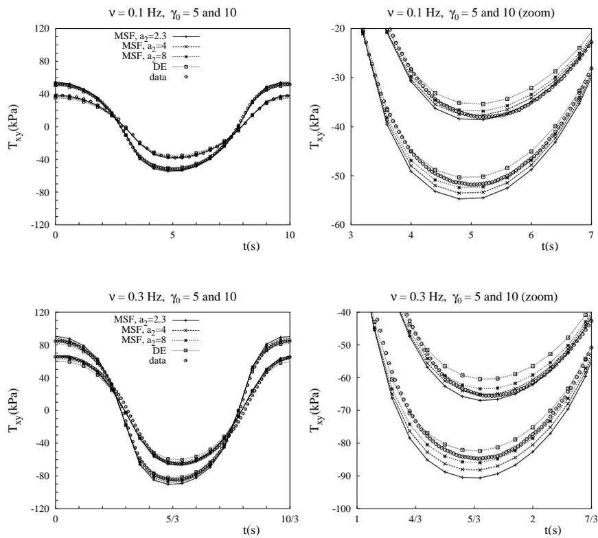
Figure A.9: Comparison of MSF model using values of  $a_2$  as in the legends and Doi-Edwards model with periodic shear stress data for Finathene melt [52]. Left column: one period; right column: zoom around minimum.
