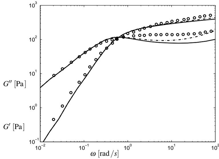
Figure 3.7: Linear viscoelastic moduli for S1. Comparison between experimental results [6](o) and the CRAFT model (—). The dashed lines are the predictions of the model for  $K_r = 3.410^{-12}$  [sDalton<sup>-2</sup>].
