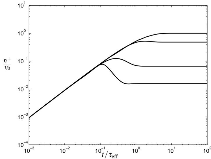
Figure 3.5: Transient shear viscosity for four different Deborah numbers. From the top, the respective Deborah numbers are 0.01, 1, 10 and 100. The finite extensibility parameter  $b$  is set to 100 and  $\tau_d/\tau_r = 30$ .
