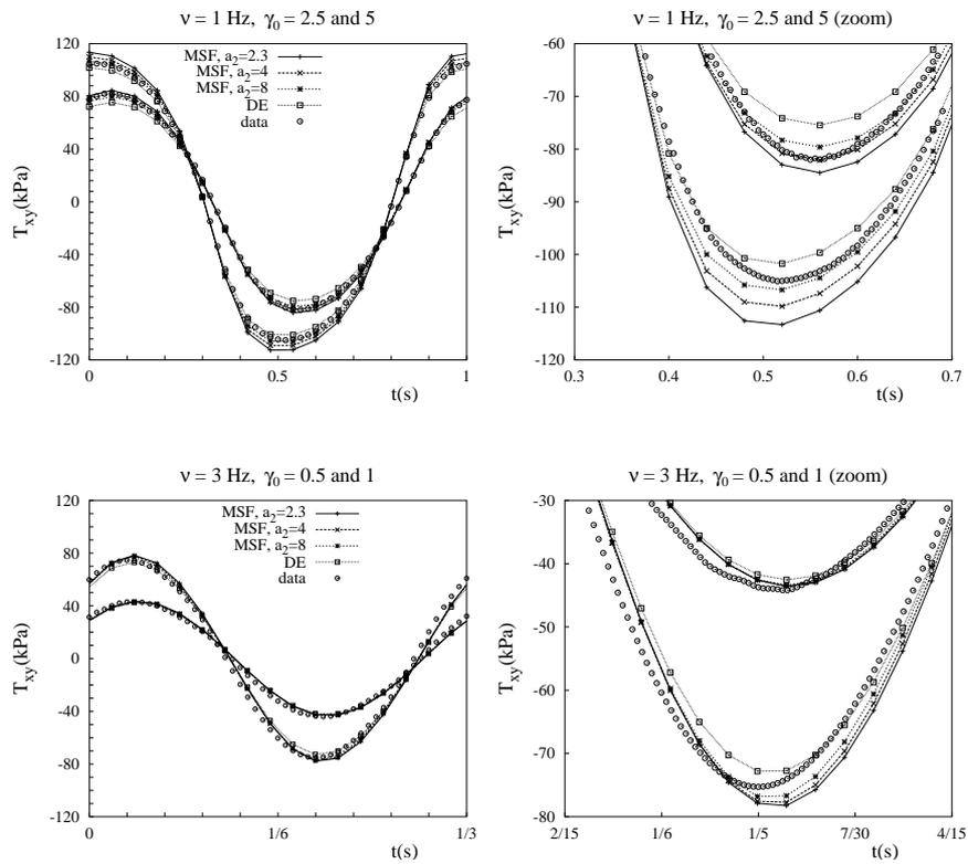
Figure A.10: Comparison of MSF model using values of  $a_2$  as in the legends and Doi-Edwards model with periodic shear stress data for Finathene melt [52]. Left column: one period; right column: zoom around minimum.
