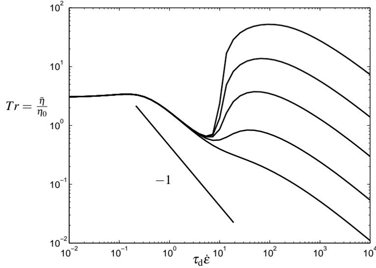
Figure 3.6: Steady state Trouton ratio for  $\tau_d/\tau_r = 30$  and different values of the finite extensibility parameter  $b$ . From the top, the respective values of  $b$  are 1000, 300, 100, 30 and 10.
