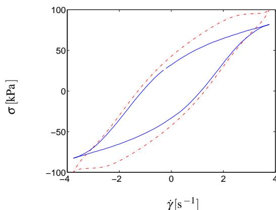
Figure 4.12: Experimental results and model predictions for PS3 at 0.1 Hz and a maximum strain of  $\gamma_0 = 6$ . The finite extensibility parameter has been reduced to  $b = 12$ . Plain line is the experimental results, the dash-dotted line is the model predictions.
