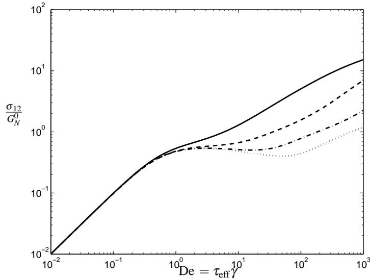
Figure 3.4: Steady state shear stress as a function of a Deborah number. The four curves correspond to different  $\tau_d/\tau_r$  ratios (—: ratio= 10, - - : ratio= 30, - · - : ratio= 100, · · · : ratio= 300). The parameter  $b$  is set to  $b = 100$ .
