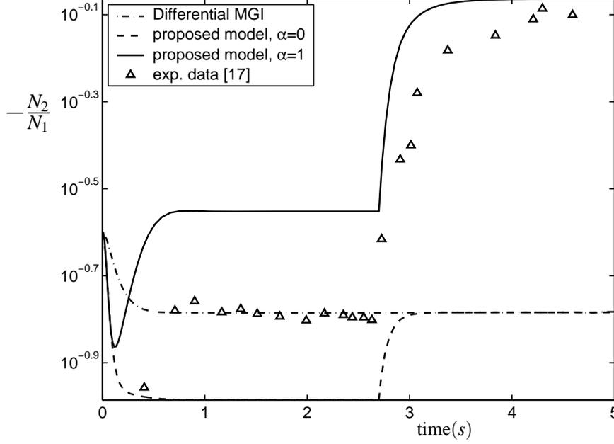
Figure 5.7: Transient normal stress ratio as a function of time. As reported in [64], a strain rate of  $20s^{-1}$  is applied between time  $0s$  and  $2.7s.$ , and  $\tau_d = 0.25s.$
