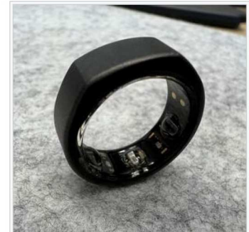
A generation 3 Oura Ring, showing some of the sensors on the inside of the ring
