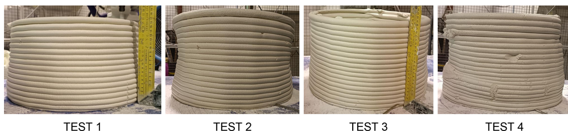
Figure 3.19 – 3D Printed Cylinders Using Different Heating Methods
