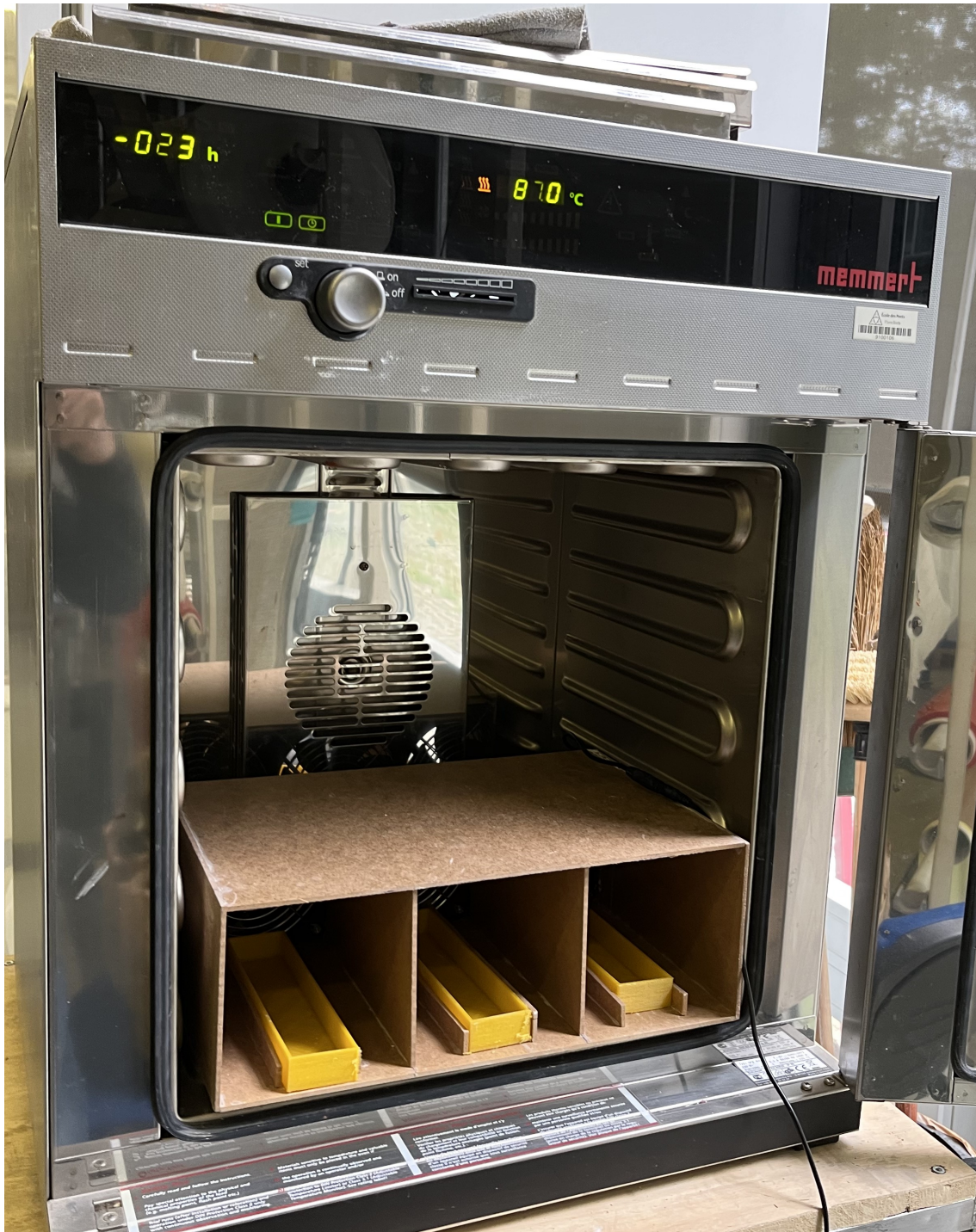
Figure 3.12 – Fabricated Wind Tunnel Inside an Oven
