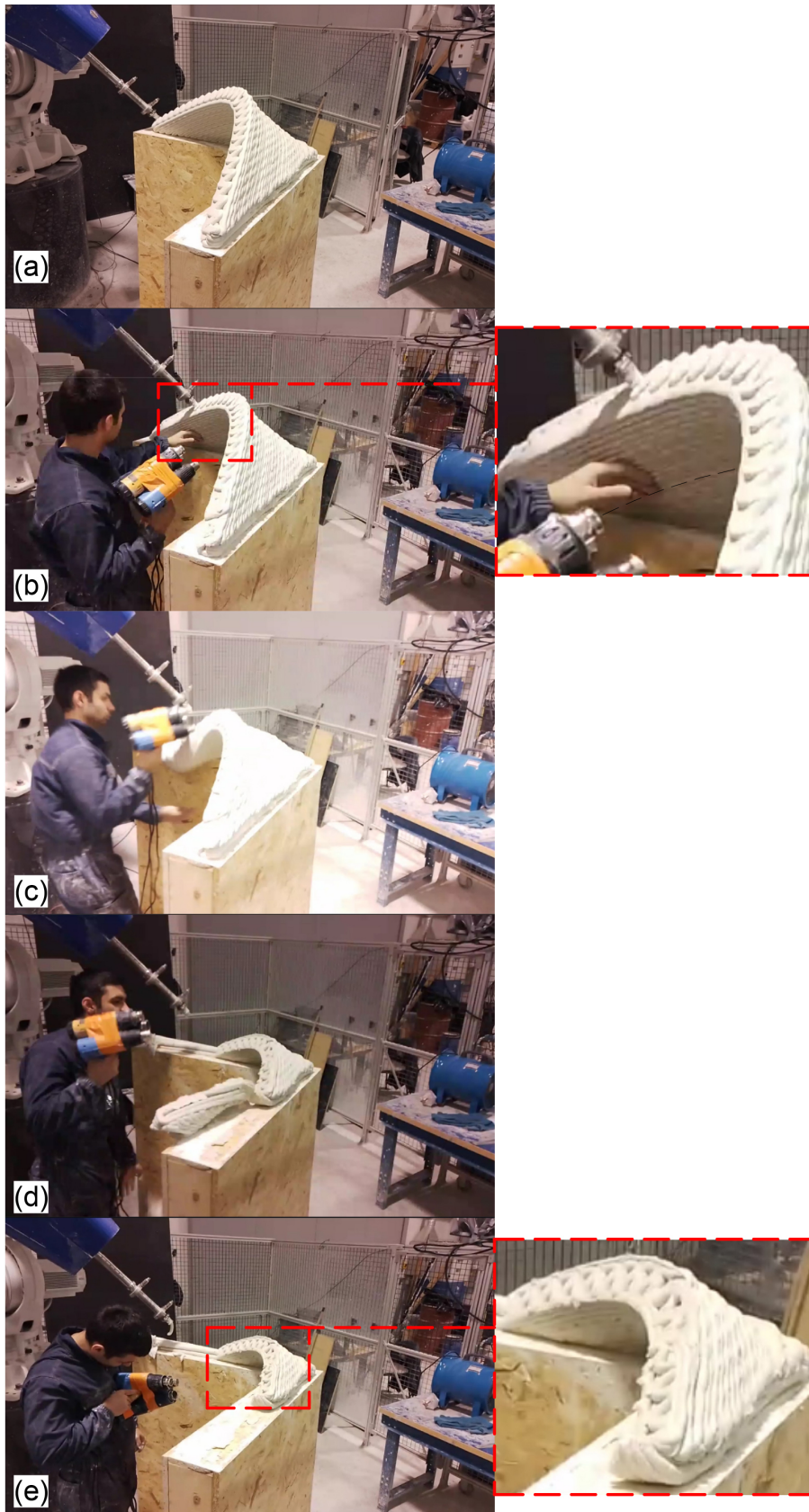
Figure 4.20 – Print Process of the Squinch with Straight Crest
