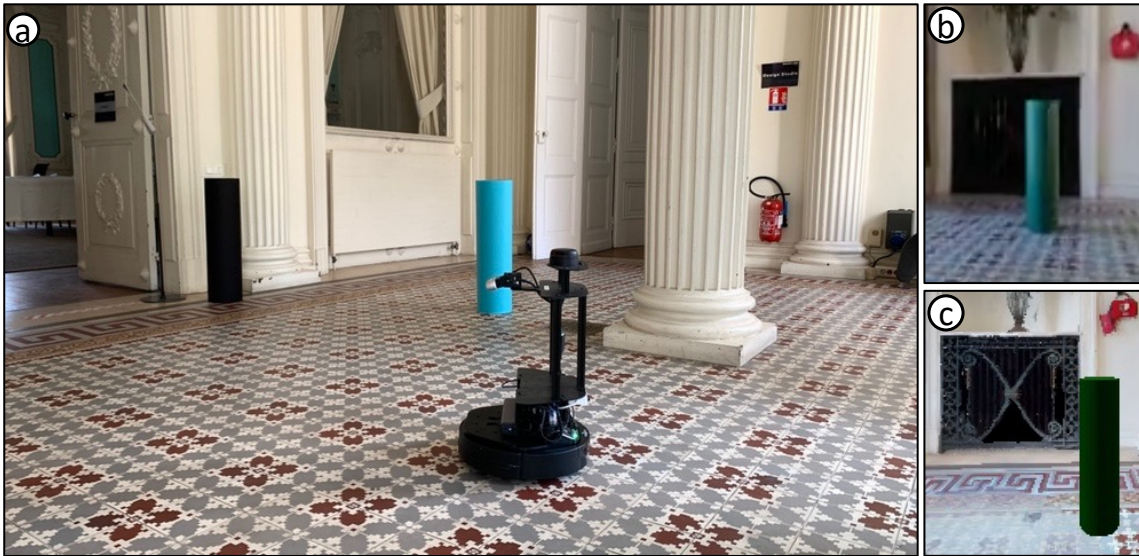
Figure 4.1 – We perform Multi-Object Navigation (Wani et al. 2020), i.e. the sequential visual search of multiple object in a given order, and are the first to do this in real physical environments (a) characterized by a large sim2real gap. This is illustrated by two first-person views (b), real and (c), simulation. We propose a hybrid method combining classical mapping and deep learning, and compare to the SOTA methods on this task using end-to-end RL training and auxiliary losses (Marza et al. 2022).
