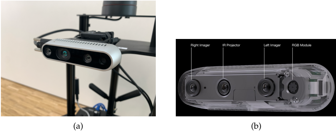
Figure 2.3 – RealSense Depth Camera : (a) Intel RealSense Depth Camera mounted on LoCoBot (Figure 2.2a). It's composed of four main modules (from left to right): Right Imager, IR Projector, Left Imager and RGB Module.
