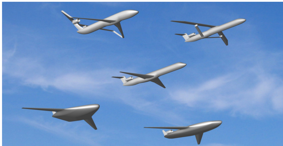
Figure 1.2: Unconventional aircraft configurations, clockwise from top left: box-wing configuration, strut-braced-wing configuration, lifting-fuselage configuration, and hybrid-wing-body configuration [17].
