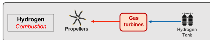
Figure 7.9: TP-H2B : Hydrogen gas turbine architecture
