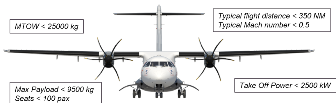
Figure 4: Main characteristic of a twin-propeller regional aircraft.
