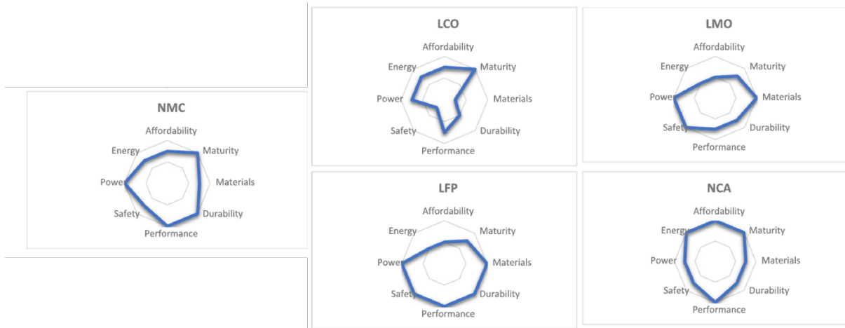
Figure 1.12: Main characteristics of commercial Li-ion batteries [33].
