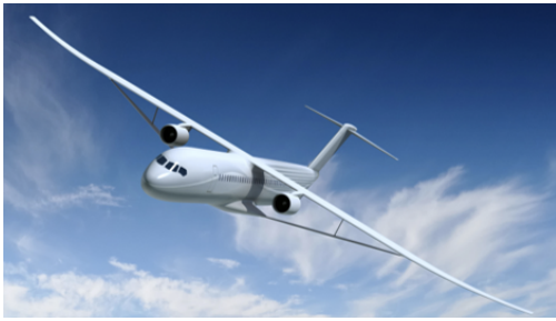
(a) Strut-braced high-aspect-ratio wings, from [49]
