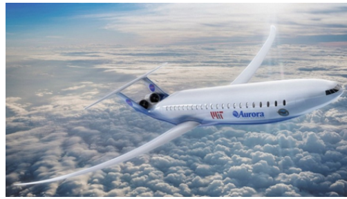
(b) Double-bubble fuselage, high-aspect-ratio wing configuration, from [54, 55]
