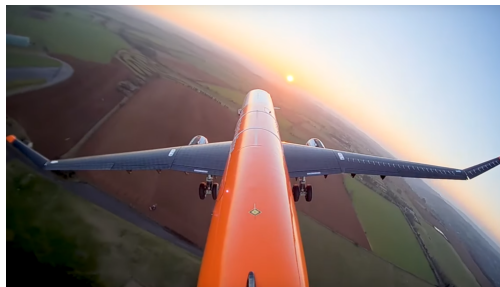
(c) Airbus AlbatrossONE semi-aeroelastic hinged wing tips, from [53]
