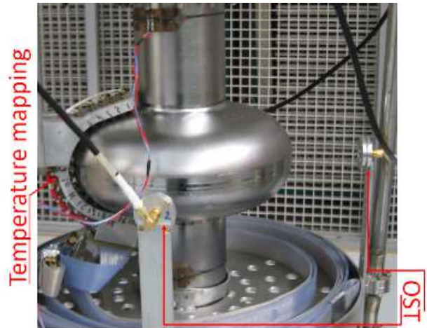
FIG. 1. 1.3 GHz single-cell cavity equipped with temperature mapping system and OSTs.
