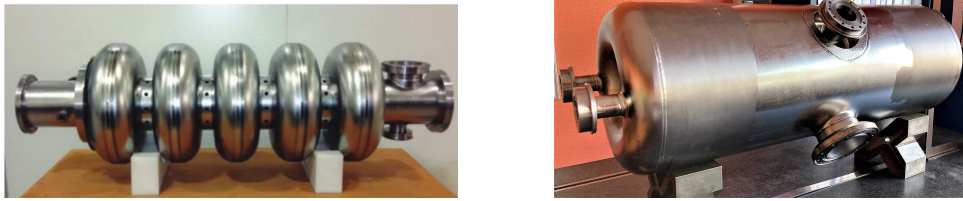
Figure 2.10: Left: picture of an ESS high beta cavity. Right: picture of the IFMIF/DONES high beta prototype.
