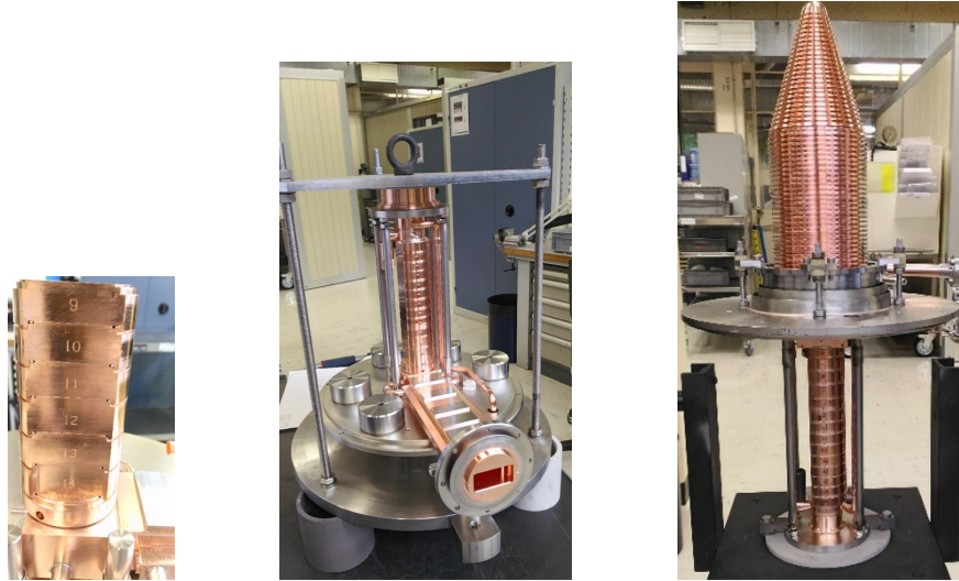
Figure 4.5: Prototype kladistron at different fabrication phases. Left: Partial cavity assembly. Center: Interaction line and output wave guide ready for brazing. Right: Tube closed.
