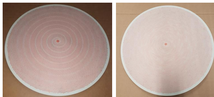
Figure 4.34. Representation of the two manufactured metasurfaces. (a) Broadside RHCP metasurface. (b) Four-beams metasurface.
