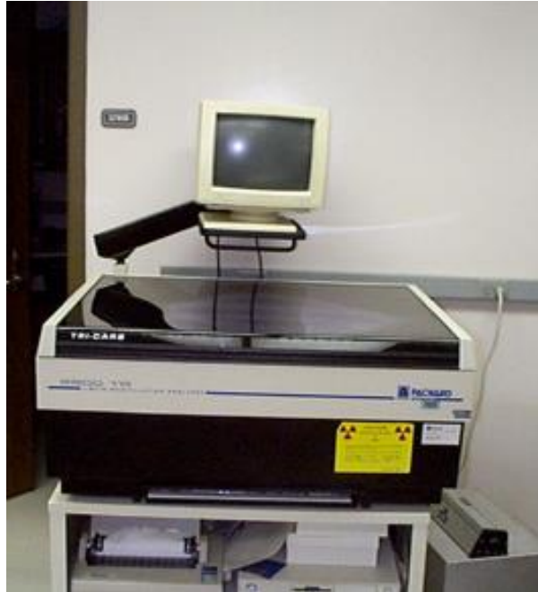
Figure 12 : Model of liquid scintillation analyser used to measure specific activity in the soils and plant samples
