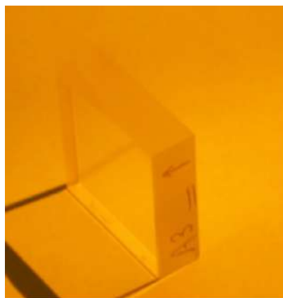
Figure 4.2: Photograph of the final gratings of the second batch with dimensions 20 \times 20 \times 6 \text{ mm}^3 after the fabrication process by Zeiss.
