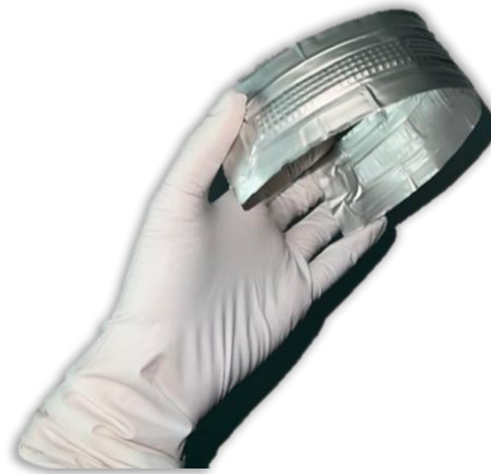
Fig. 5.10. The fabricated flexible polymeric TGP.
