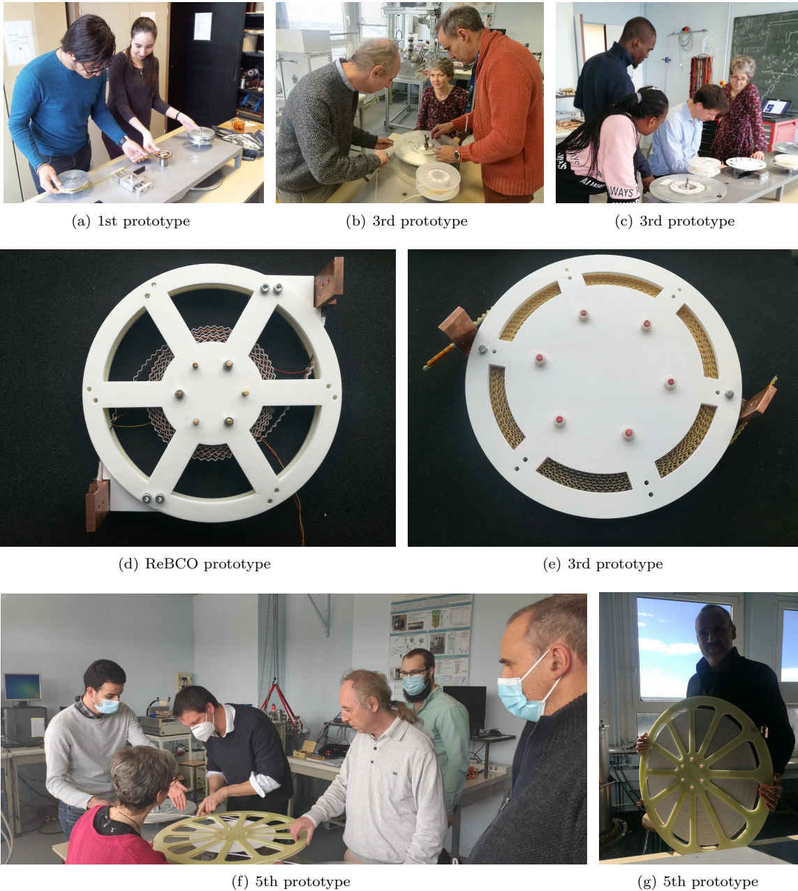
Figure 4.21: Winding of the ScPF prototypes at GREEN Laboratory, Nancy (Jan. 2020-Apr. 2021).
