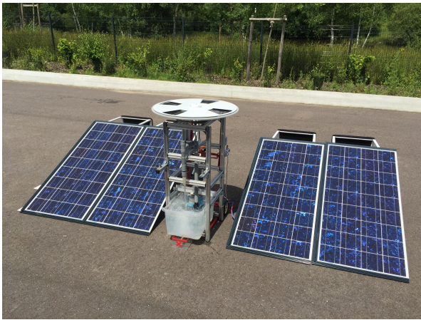
(c) First PVWPS with SAUREA's motor and a centrifugal pump in 2016.
