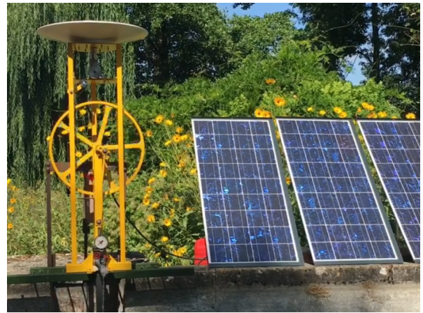
(d) First PVWPS with SAUREA's motor and a mini-Volanta piston pump in 2019.
