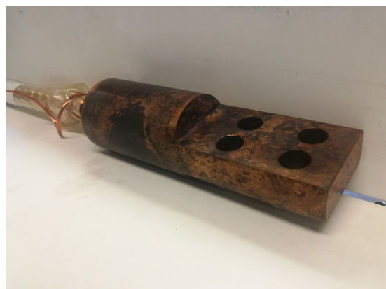
(f) Current lead soldered to the HTS cable
