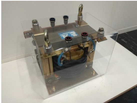
(a) 800 A step down transformer
