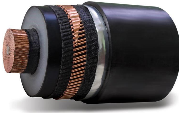
Figure 3.5: HVAC resistive cable: single core copper conductor, XLPE insulated, copper wire screen and HDPE sheath [73].
