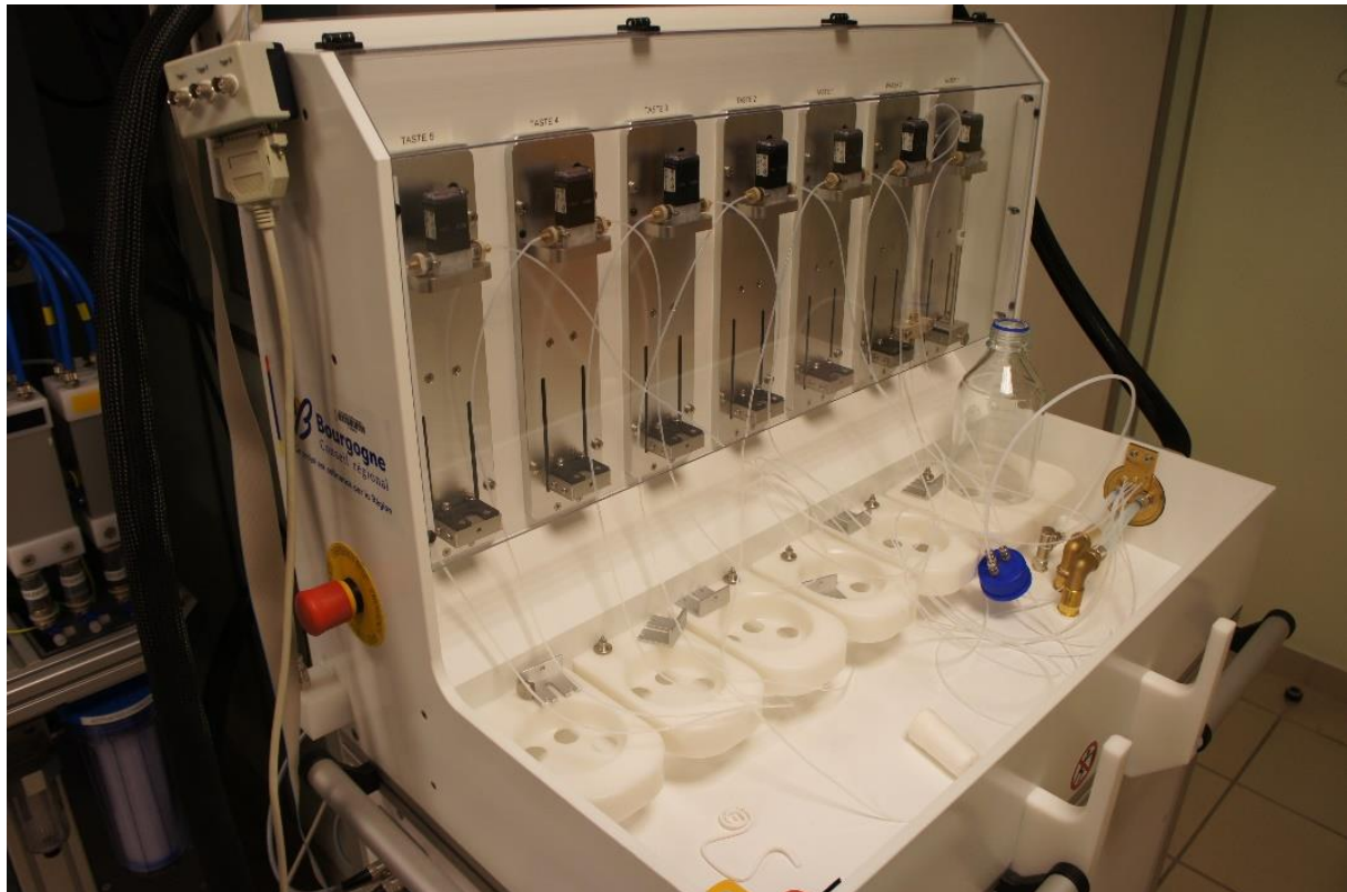
Figure 32. Gustometer model Burghart GU002.
