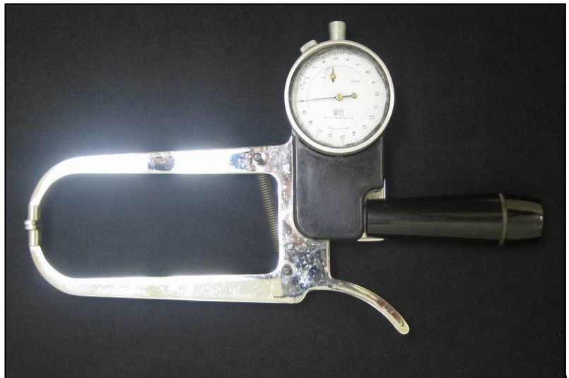
Figure 3. Calipers, tool for the diameter and deformability.
