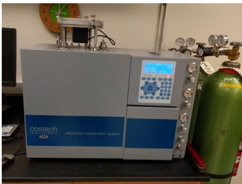
Figure 3.8: Costech ECS4010 elemental combustion system used for C and N measurements at the GRiTS laboratory, Earth and Environmental Sciences Department, University of Michigan, USA.
