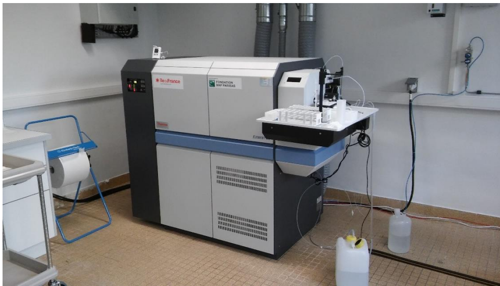
Figure 3.7: ThermoScientific Element XR-HR-ICP-MS at GEOPS, France. Photo curtesy of Frédéric Haurine.
