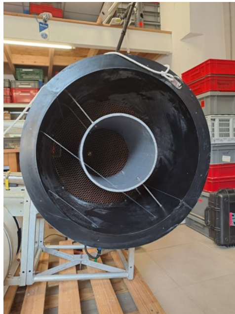
Figure S4.4: View inside the VisuTrap once the top honeycomb mesh is removed. The bottom honeycomb mesh stands above the UVP6 field of view. The PVC tube joins the two honeycomb meshes and reduces the trap aspect ratio.
