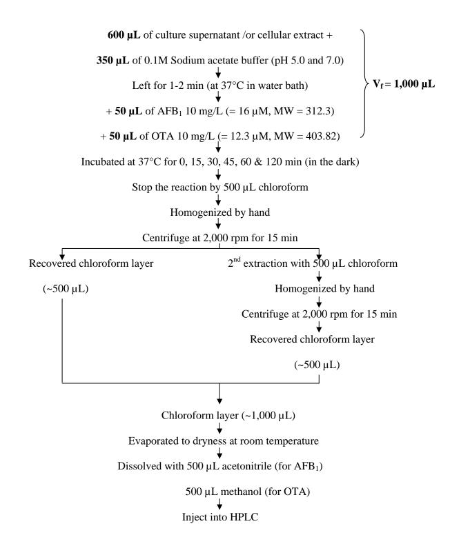
**Fig. 5.2** Summarized diagram for kinetic degradation of AFB<sub>1</sub> and OTA by culture supernatant /or cellular extract from both *Bacillus* CM 21 and *Bacillus* MHS 13.
