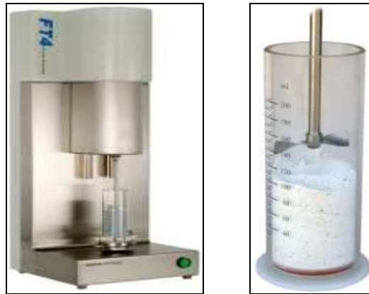
Figure II.15. FT4 Powder Rheometer (Freeman, 2006)
