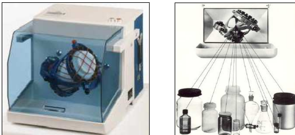
Figure II.4. Turbula Mixer (Chéry et al., 2007)
