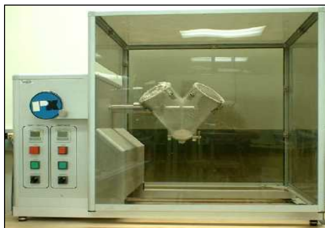
Figure I.21. V-Blender (Yang et al., 2005)
