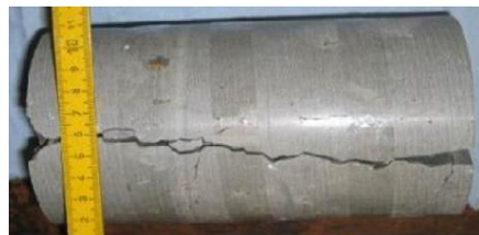
Figure 5.32. Cracked CO x sample by Brazil splitting test (Zhang, 2013)
