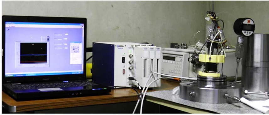
Figure 5.3. The setup (LVDT) of gas injection and water injection tests (Davy et al., 2007)
