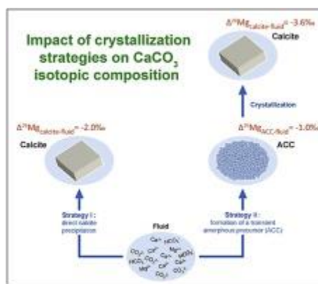
Figure 51. An example of geochemical differences between calcite precipitated directly from the fluid, or through an ACC precursor (Mavromatis et al., 2017)
