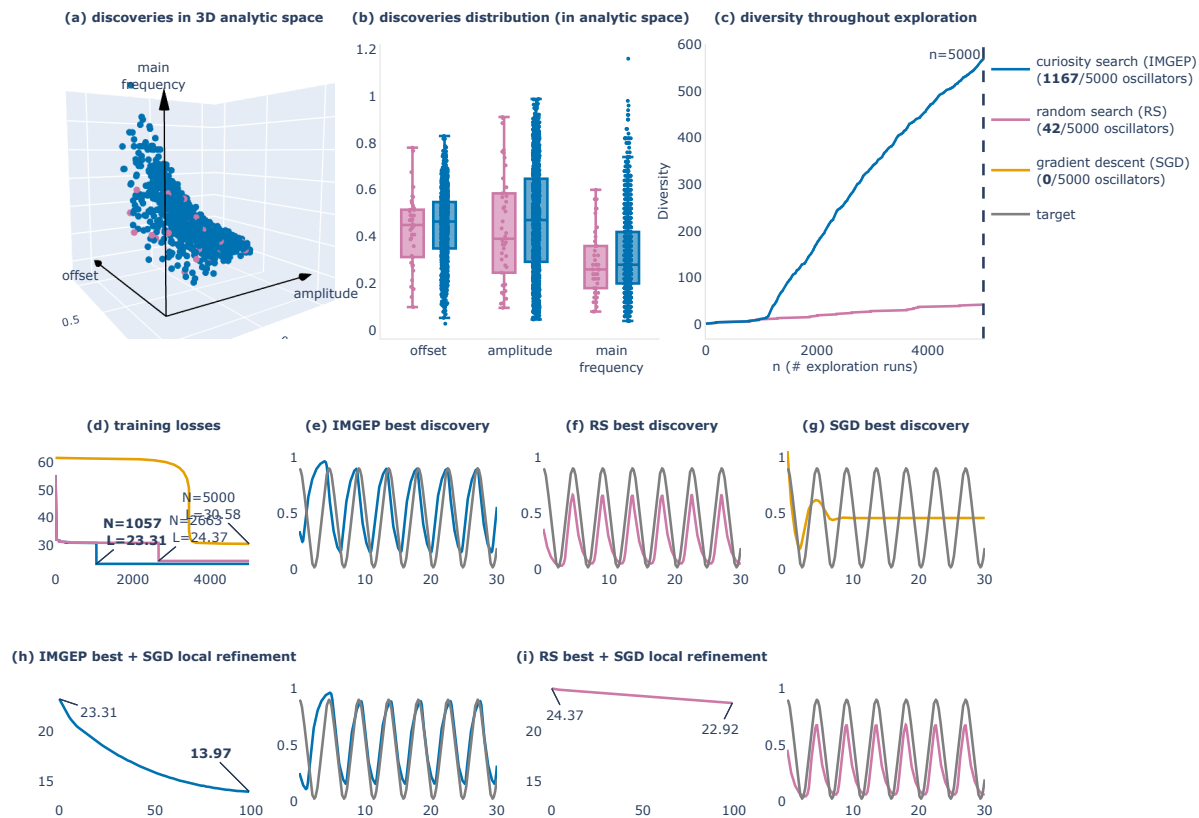
Figure 8.10. Comparison of three alternative strategies for the design of oscillator circuits: curiosity search (blue), random search (pink), and gradient descent (orange). (a-c) Given a budget of 5000 experiments, curiosity search is able to find 1167 oscillator circuits (ones showing sustained oscillations), whereas random search only finds 42 oscillators and gradient descent does not discover any (starting from a single random initialization). (a) 3D scatter plot of the 42 random search discoveries (pink) and 1167 curiosity search ones (blue) in the (amplitude, main frequency, offset) analytic behavior space. (b) Box plots projecting points from the 3D scatter plot into the respective (amplitude, main frequency, offset) axes. (c) Diversity discovered throughout exploration, where diversity is measured with a binning-based space coverage metric (20 bins per dimension). (d) Evolution of the training loss L for the three exploration strategies. (e-f-g) Corresponding best discoveries (for which L is minimal) for the three exploration strategies. (h-i) Local training loss and resulting finetuning of the best discoveries with gradient descent.
