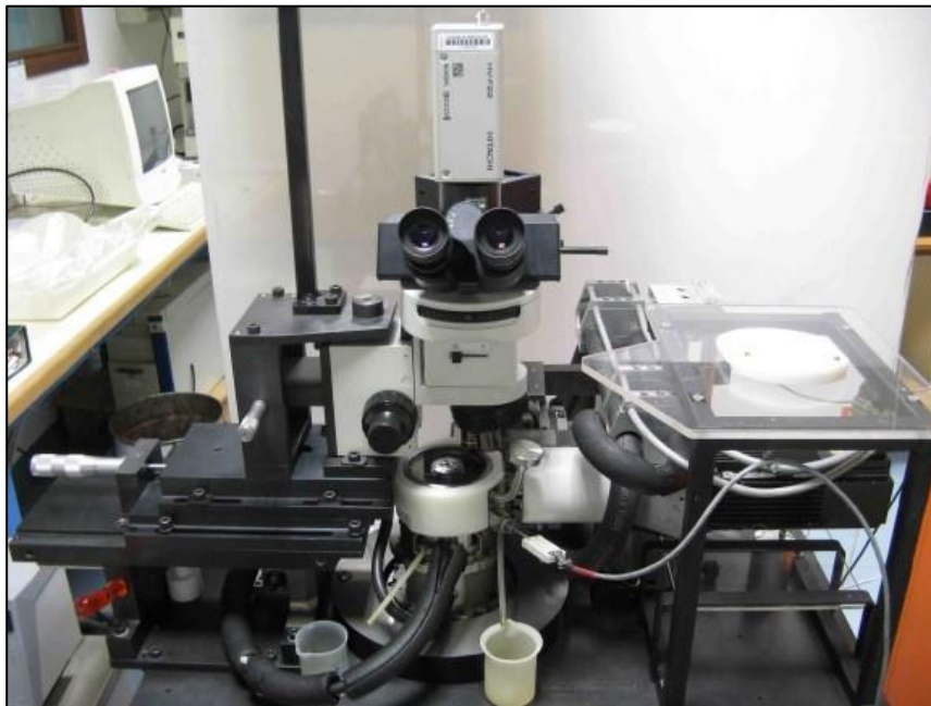
Figure 2.4. Jerotrib test rig.
