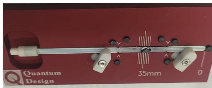
Figure 2. 11: Photograph of VSM-Oven mode used for high temperature measurement, LPMC Amiens, France.
