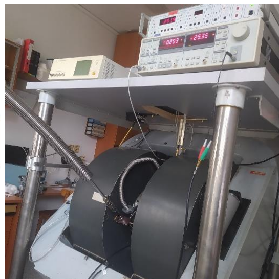
Figure 2. 15: (a) Schematic of device for measuring the magnetoelectric effect, (b) Photograph of device for measuring the magnetoelectric effect used in FZU, Prague, Czech.
