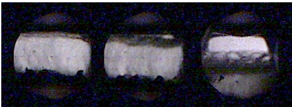
Figure 2.3: Visualisation of the phase separation of water occurring at 200 bar/365°C. Top and bottom pistons are visible, the sample is between the pistons in the clear area.
