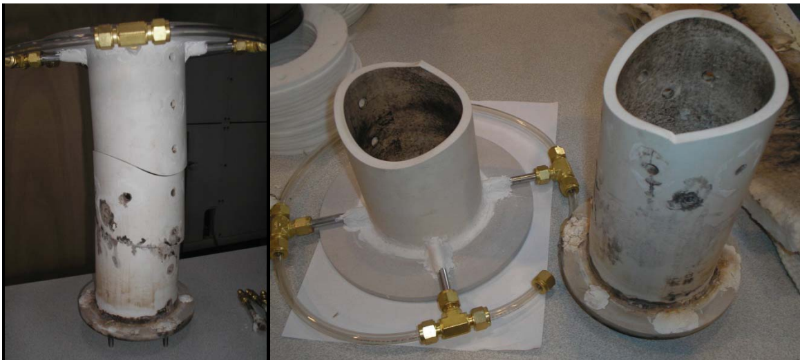
Figure (IV-16) - Photograph of the mullite reactor after the first experiment.
