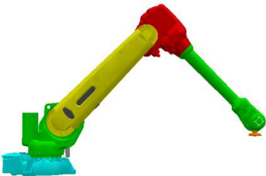
(a) Configuration elbow(up)- shoulder(right)-wrist(unflip)
