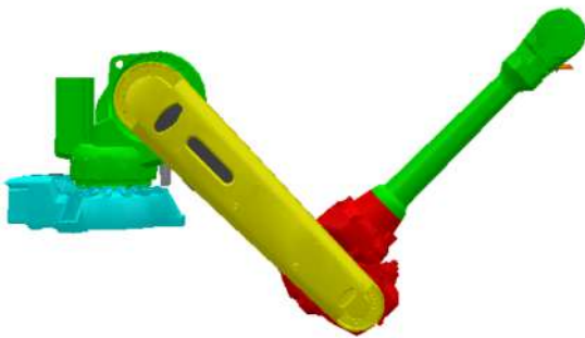
(e) Configuration elbow(down)- shoulder(right)-wrist(unflip)
