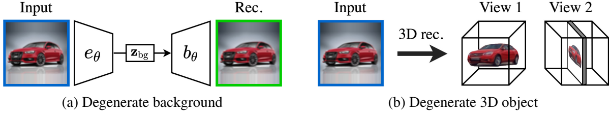
Figure 5.4: Degenerate solutions. An SVR system learned by raw image autoencoding is prone to degenerate solutions through (a) the background or (b) the 3D object model. We alleviate the issue with cross-instance consistency.
