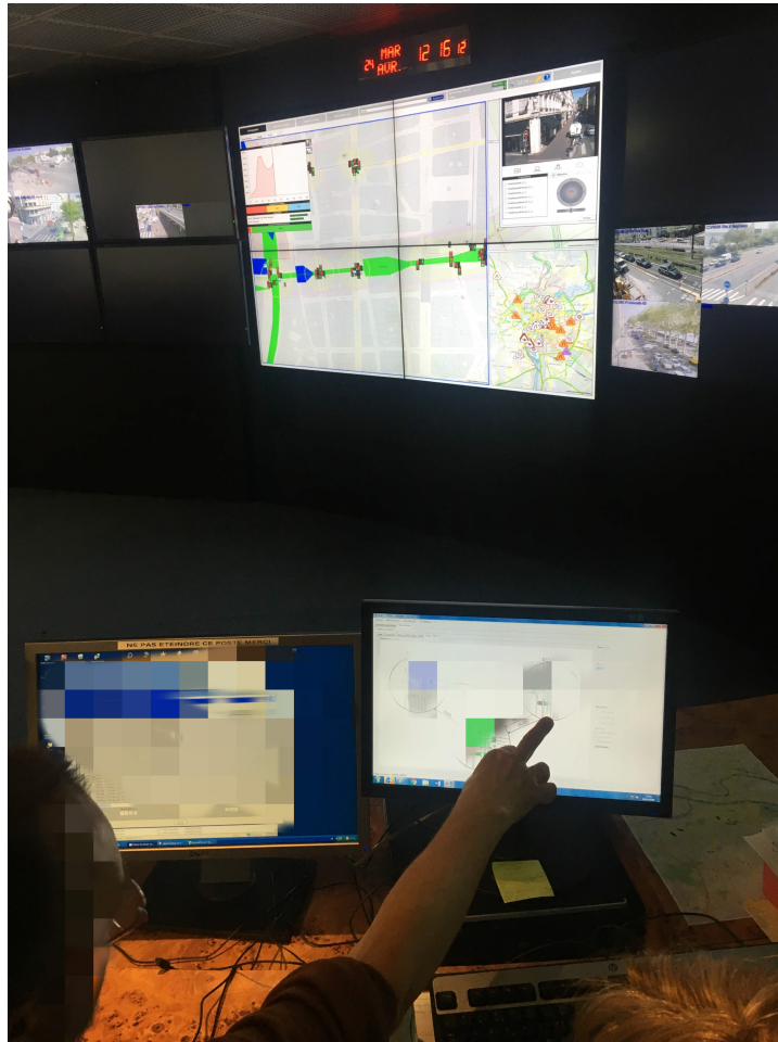
Figure 6.1: A picture we took in the traffic control center in Lyon, France, an indoor physical facility where operators monitor traffic on a large display from remote workstations. It offers the visual environment for merging multiple visualization techniques to analyze heterogeneous spatio-temporal traffic data.
