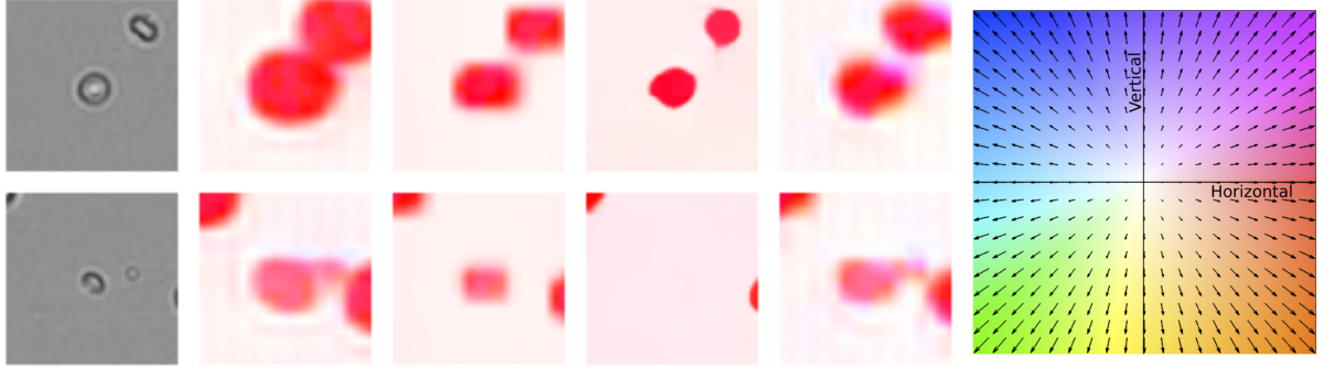
Figure A.4 – Comparison of all flow models evaluated in the chapter. First column is a random sample of cells in the sequence, retrieved at the same timestep (first image of the RBC sequence). Second column is the unregularized UFlow model. Third column is UFlow regularized with first-order smoothness. Fourth column is RAFT, and last column is UFlow regularized with Sparse Variation.
