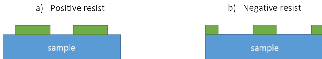
Figure 111. Sketch of the sample after development. a) In the case of positive resist. b) In the case of negative resist.
