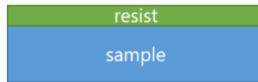
Figure 109. Sketch of the resist spread evenly over the surface of the sample after spin coating.
