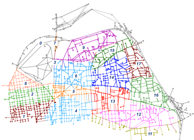
Figure 5.16: The northern region network of the conurbation of Lyon (3rd, 6th district of Lyon and Villeurbanne). The network contains 1,883 nodes, 3,383 links and is divided in 17 zones. Each zone is represented by a distinct colour.
