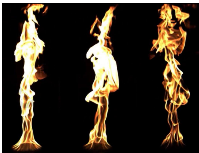
Figure 3.2 – Real view of the three experimented flames, with decreasing X_{O_2} from left to right, Zeng et al. (2019).
