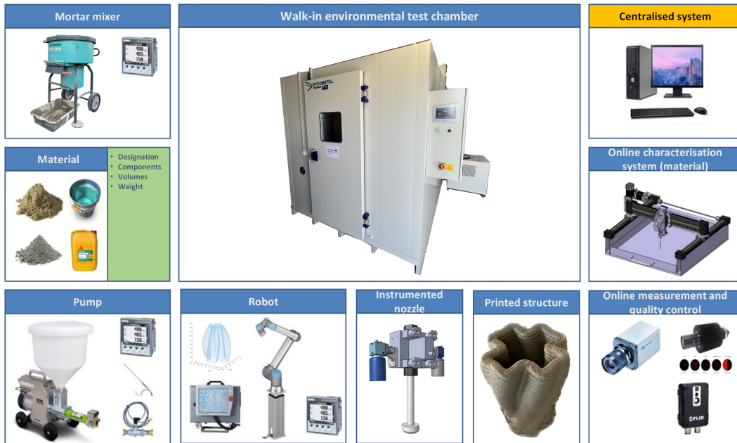
Figure 7.1: Online measurement and data collection system for creating digital twin for 3D concrete printing.
