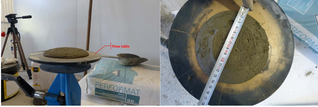
Figure 3.19: Flow table test to determine the workability of fresh concrete.
