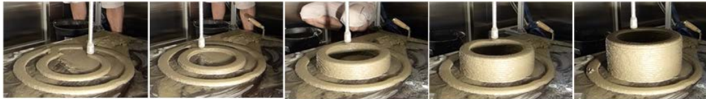
Figure 2.3: Building up a cylindrical structure layer by layer.
