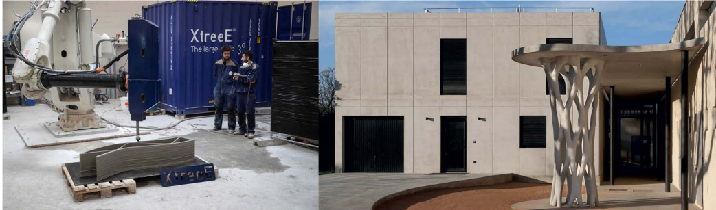
Figure 2.11: The printer developed by XtreeE using an ABB industrial manipulator.
