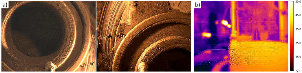
Figure A.2: Time-stamped image data sample captured during printing test under T = 10^{\circ}\text{C} . a) RGB images of freshly deposited filament from top-view captured by two cameras integrated on the nozzle. b) Thermal image captured by the thermal camera placed in front of the printed object.
