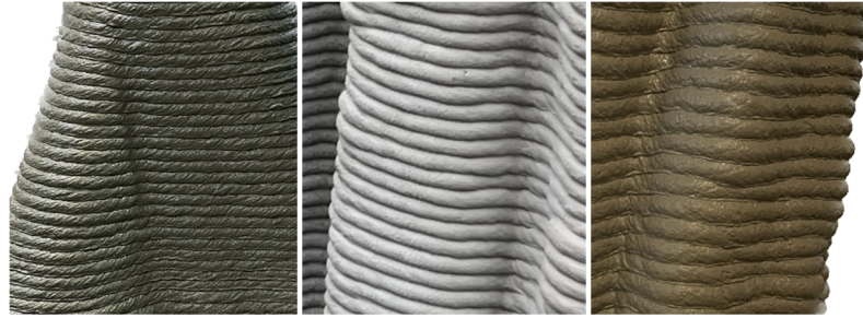
Figure 4.28: Layer height considered constant across the printed shape.
